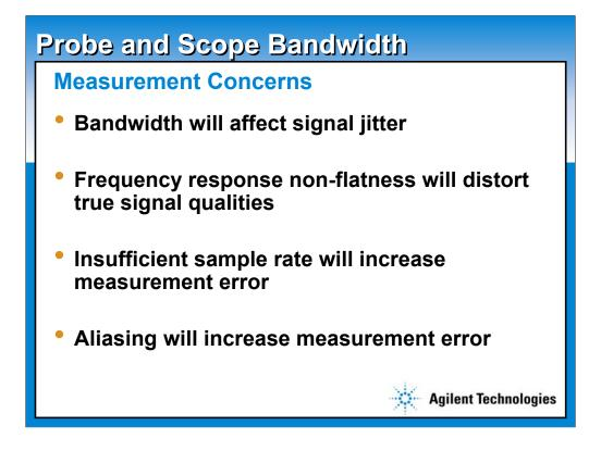
In this section, we will look at the effects of system bandwidth on jitter measurements and their relative accuracy. We will address the issues of flatness in the frequency response of the scope, probes and/or cabling used to connect to the target system, and insufficient sample rate that may cause aliasing of the target signal.
