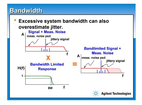
It is also possible for the measurement system bandwidth to be too high. If the measurement system noise floor dominates the error of a jitter measurement, and the measurement system has excessive bandwidth, then reducing the system bandwidth may produce a more accurate answer by reducing the jitter measurement floor.
