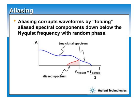
Aliasing occurs in real-time oscilloscopes if the measured signal contains spectral content above the Nyquist frequency, where the Nyquist frequency is one half of the oscilloscope's sampling frequency. Aliasing distorts sampled waveforms by "folding" the aliased spectral components of the signal down below the Nyquist frequency with random phase.
