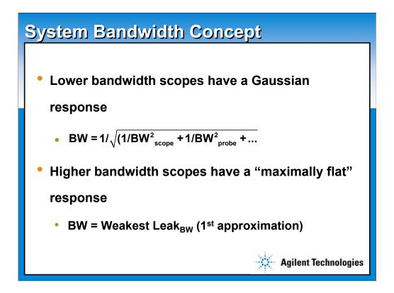
Lower bandwidth oscilloscope systems (<=1GHz) typically have a Gaussian frequency response. In a Gaussian-type system, bandwidth can be computed using the familiar square root of the sum of the squares formula, where the frequency response of the 'system' will behave as a series of cascaded low-pass filters with slow rolloff characteristics:
