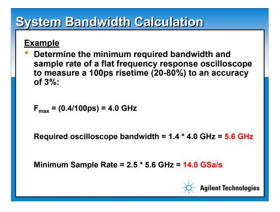
Many of today's high-speed buses and chip-to-chip signals have rise time specifications in the 100ps range (20% to 80%) as shown earlier. So, let's go walk through an example of accurately measuring a 100ps edge.
