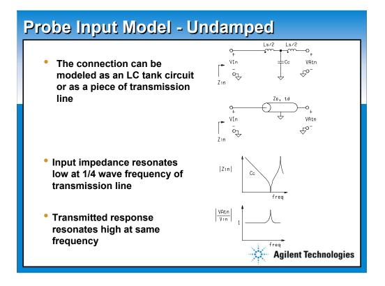
With the assumption of minimized ground lead connections, the model of our input connection begins to look like a single transmission line (as opposed to coupled lines). And that is exactly what it is! This model of the probe connection dominates the performance of the oscilloscope system. In most cases, you can assume that the model for the probe amplifier and oscilloscope are perfect (infinitely flat response).
