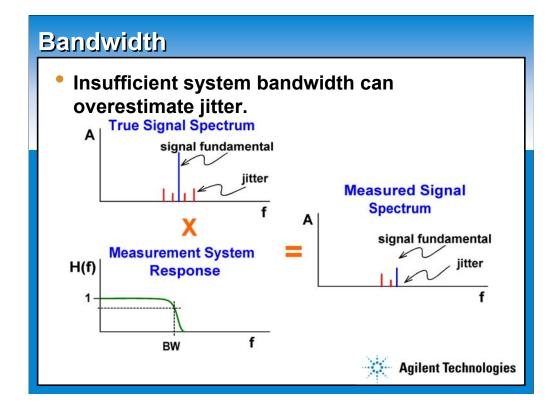
The effect of bandwidth on jitter measurement accuracy can be a complex issue. Just because the bandwidth of one measurement system, including probes or cables is higher than another one, doesn't mean it will always produce a more accurate answer.
