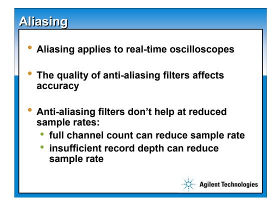
Most oscilloscopes employ fixed-bandwidth analog anti-aliasing filters in front of their analogto-digital converters (ADCs). These filters reduce the magnitude of the signal spectra that can be aliased by the sampling process at the maximum sample rate. Some anti-aliasing filters provide better protection against aliasing than others, and this matters when the measured signals push the bandwidths and sample rates of the oscilloscopes.
