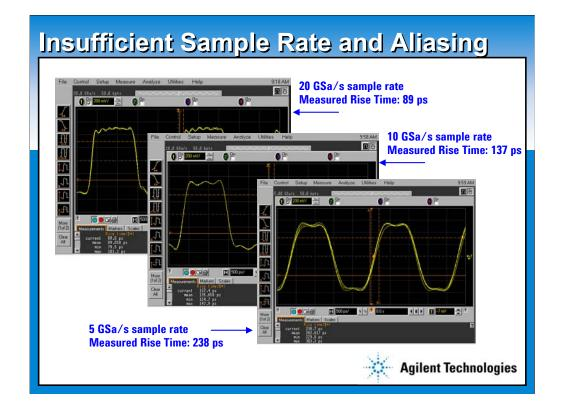
To illustrate the point of better accuracy with higher sample rate, this slide shows the same high-speed signal captured at three different sample rates. The measured rise times of this signal vary significantly depending upon the sample rate. So the caution here is, watch out for scopes that trade-off sample rate for channels. Many high-bandwidth four channel scopes only sample at the highest specified rate (banner spec) when using just one or two of the acquisition channels.
