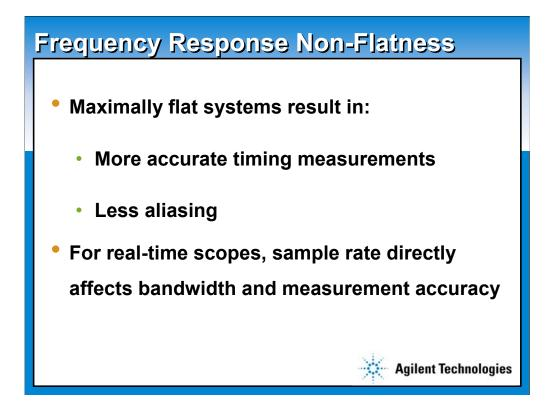
Maximally flat systems typically result in better timing measurement accuracy. If the input signal under test is band limited, then the maximally flat systems captures more of the higher frequency components of the signal up to the bandwidth (-3dB). For high-speed signals in the 100ps edge range, this is the case.
