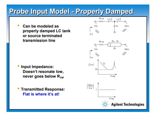
In the past the only way to keep the frequency of this resonance above the bandwidth of the probe was to use an ultra-short, stubby point at the input of the probe. Although this produces good high frequency fidelity, it is often difficult to connect such a short blunt point to the circuit.
